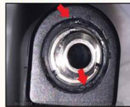
Photo 2. Scratches and gouges surrounding channel port
