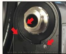
Photo 1. Channel port with rusty discoloration; oily deposits and white, foamy residue near port
